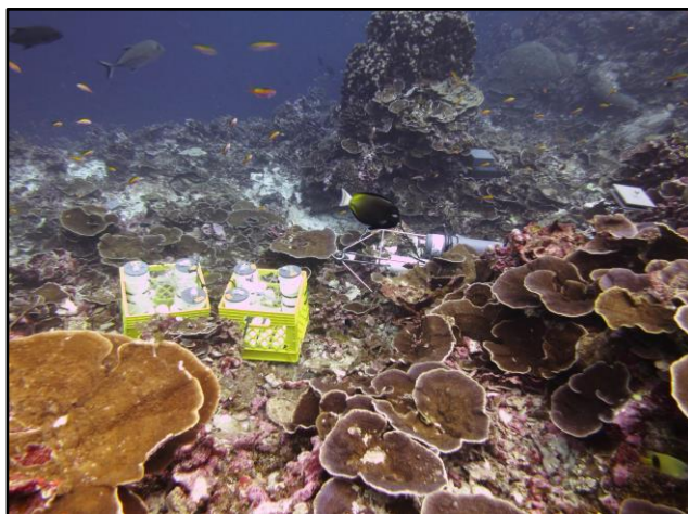
1086 1087 Figure 2-7. Short-term and long-term moored instruments deployed at Jarvis Island by the NOAA Pacific Islands Fisheries 1088 Science Center. The yellow crates are the temporary deployment (1-3 days) of water sampling units) and the CTD and pH 1089 sensors (in the metal cage). The Calcification Accretion Unit and an Autonomous Reef Monitoring Structure (the square 1090 structures) towards the right in the photo are the longer-term deployments (~3 yrs). Source: NOAA Pacific Island Fisheries 1091 Science Center
